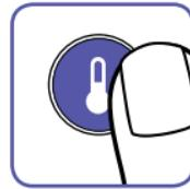
When the temperature button is pressed a dashed line animation will appear on the screen. **DO NOT** remove thermometer from forehead until you hear a long beep indicating normal temperature range or 10 short beeps indicating fever.
