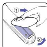
Replace the batteries when the flashing battery symbol appears on the LCD screen.
