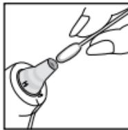
Once the alcohol has dried completely, a new hygienic lens filter can be put on and a temperature measurement taken. If the probe tip is damaged, please contact your authorized local service center.
