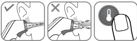
**6** ExacTemp® Stability Indicator light will pulse while temperature measurement is in progress. The light will remain solid for 3 seconds to indicate that a successful temperature reading has been achieved.
