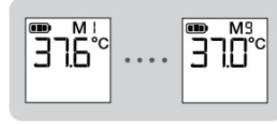
Memory mode is automatically exited by not pressing the memory button for 5 seconds.
