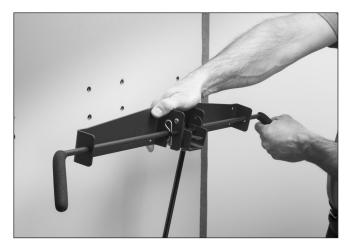
Secure the pneumatic cylinder's bracket to the backrest with the (8) eight 3/4" pan head screws.
