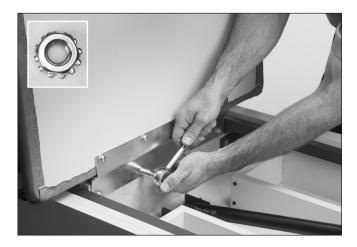
2 Extend the pneumatic cylinder about half way by holding the apparatus with one hand and pressing down on one of the levers with the other.
