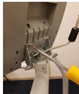
Slide slots onto tabs in bracket
