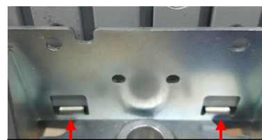
Slide slots onto tabs in bracket
