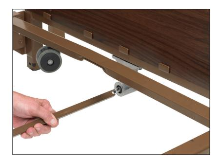
12. Install the head end of the shaft as shown.
