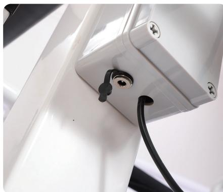
Pull down the dust cap located at the bottom left side of the Control Box.
