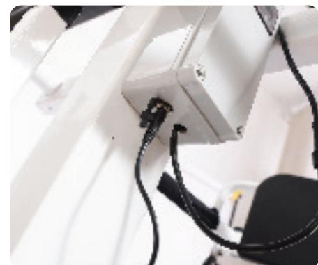
Connect the Power Adapter to the charging port on the left side of the Control Box.
