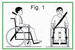
Restraints should make direct contact across the front of the body and in the area where the thigh and pelvis meet.
