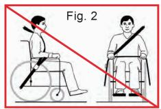
Do not allow belt restraints to wrap around or over wheelchair components as this will keep them from fitting securely across the body.
