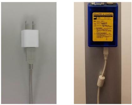
4. Connect the USB Wall Power Adapter to a wall power outlet as shown.
