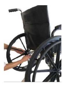
**DUAL AXLE – ADJUSTABLE SEAT HEIGHT -** Seat-to-floor height can be adjusted up or down approximately 2". The wheels & castors have several holes to allow adjusting up or down. The combination of these adjustments allow for about 2 inches of adjustment in seat-to-floor height.
