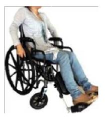
**TIRES** - Solid rubber tires need minimal maintenance, but should be cleaned occasionally with a damp cloth. Replace if tires become severely worn or cracking appears.
