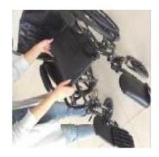
**REMOVABLE ARMS** - Remove arms by depressing spring button and lifting arms out of front and rear sockets.
