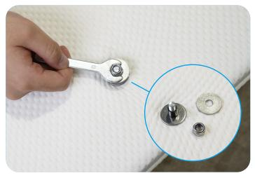
Align the screws with the holes and insert them downward into the designated holes. There are a total of 7 holes for the two mattresses combined.
