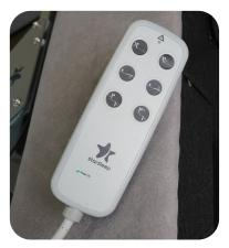
After installation, please connect the power supply. If the green indicator light on the remote control is flashing, it indicates that the ORIN bed is charging normally. Once the charging is complete, the light will automatically turn off.
